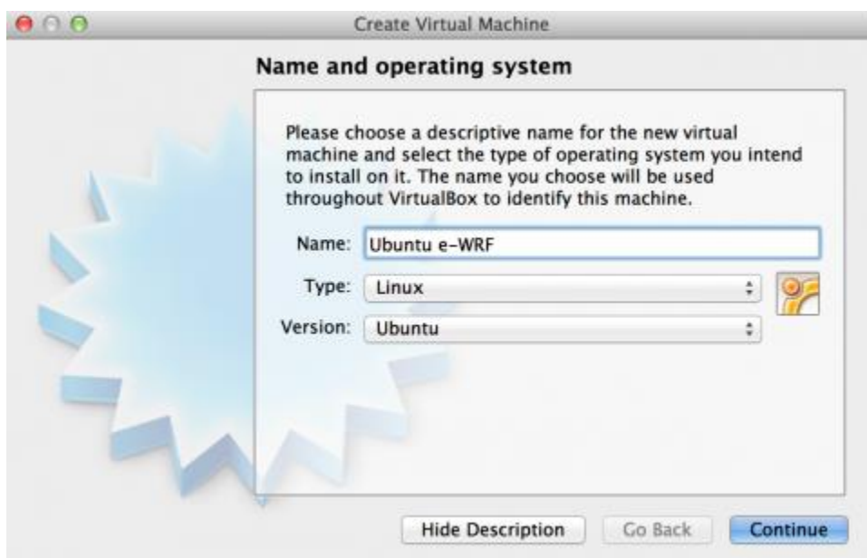
Figure 1.3 - Setting up a name for our installation. In this case, the name chosen was "Ubuntu e-WRF." Make sure the other options are selected as shown in this figure.
